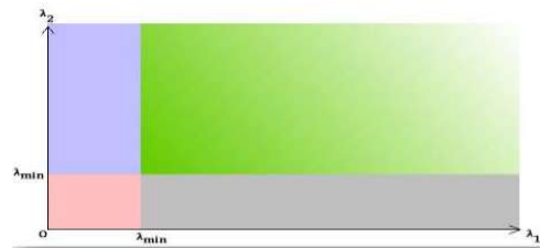
Fig. 13: Type detection according to the obtained values \lambda_1 and \lambda_2 [49].
