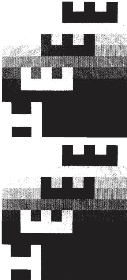
Figure 1.29 Example of phase-only reconstruction by a closed-form algorithm. (a) Original image of 12 \times 12 pixels. One pixel in the image is a large square block; (b) phase-only reconstruction of the image in (a) by solving a set of linear equations in (1.44).
