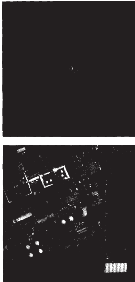
Figure 1.33 Example of the Fourier transform magnitude of an image. (a) Original image x(n_1, n_2) of 512 \times 512 pixels; (b) |X(\omega_1, \omega_2)|^{1/4} , scaled such that the smallest value maps to the darkest level and the largest value maps to the brightest level. The operation (\cdot)^{1/4} has the effect of compressing large amplitudes while expanding small amplitudes, and therefore shows |X(\omega_1, \omega_2)| more clearly for higher-frequency regions.
