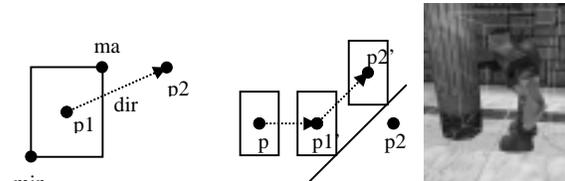
**Fig 1** AABB defined by max and min points moving from p1 to p2 (left) Collision detection/response recursion. AABB was moving from p1 to p2. Recursion continues until no collision is found (center). Results on collision detection (right)
