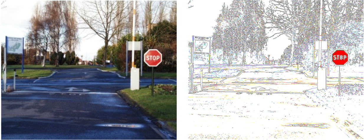
Figure 1 : (Left) Typical example of a road scene with a polygonal shape (stop sign), with edge detection [10] and color segmentation (right).
