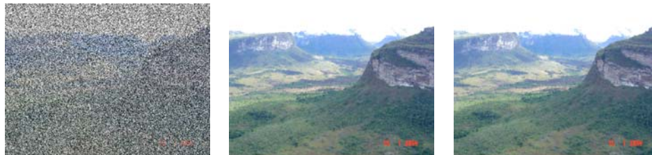
Fig. 2 Diamantina color image with 70% salt e pepper noise (left), reconstructed with Newman r=1 after 14 iterations (center) and reconstructed with Moore r=1 after 12 iterations (right)
