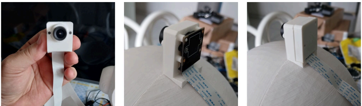
Figure 84: Images of the camera support, its mounting on the robot's head and its connection to the Raspberry PI via the flat cable.
