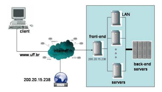
Figure 2.1: Cluster-based Web server architecture.
